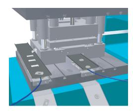
Our **SN9810** pneumatic part conveyors ensure a comfortable removal of punching- and bending waste from the production plants.
