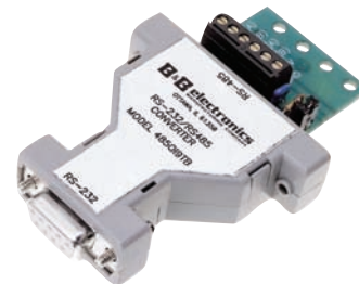
0830-0473-0005 232 to 485, Isolated, DB9 Female to Screw Terminals
