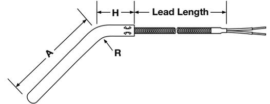
The bent rigid tube offers protection and accurate lead placement around machinery.
