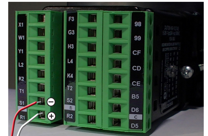
Figure 4: Thermocouple Wiring Example
