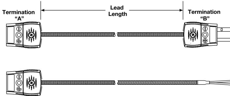
Flexible extensions allow thermocouples to be disconnected from a system without disturbing the remaining wiring.
