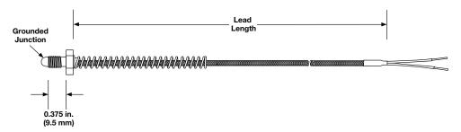
The nozzle thermocouple has a short installation depth and a low profile to allow control of thin platen sections.
